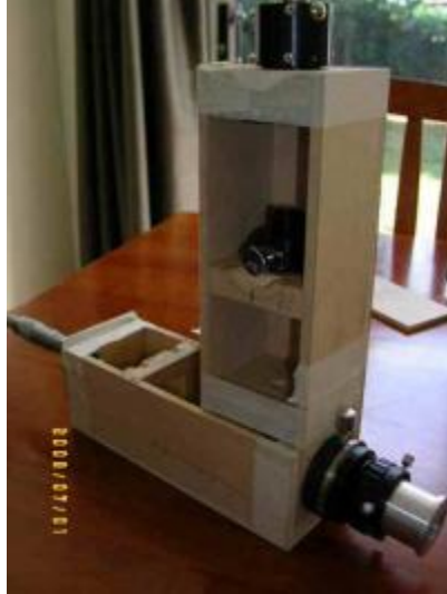
Fig 11: Construction detail – overall arrangement – slit at top RHS, eyepiece below and micrometer at LHS
