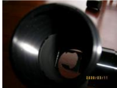
Fig 2: 50/50 Beamsplitter mounted in Meade body
