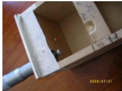
Fig 14: Grating adjusting micrometer – 6mm ball added, laser alignment dot visible on back surface of grating section
