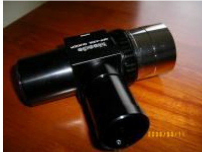
Fig 1: Modified Meade Off-axis guider body
