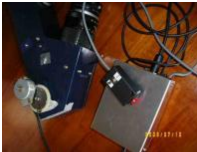
Fig 3: Stepper motor and controller for grating rotation
