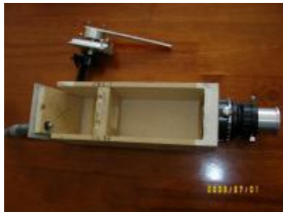
Fig 13: Collimating lens cell with square aperture, grating holder above
